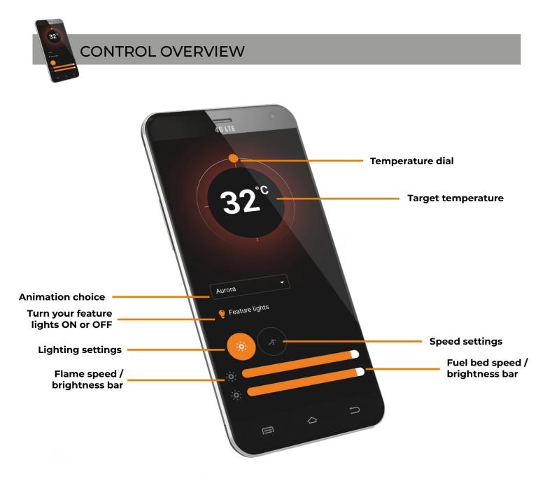
To adjust the desired temperature of your fire ensure that the heater is selected on the Home Page in the previous step. Then press, hold, and rotate the temperature dial to set the temperature.
