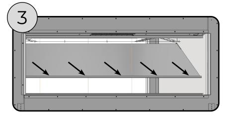
Once the glass has been inserted into the clip, ensure the bottom of the glass been fitted to rest on the retainer bar. You can then repeat the process on the other side.
