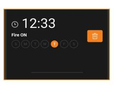
The above screen will now show your set timer. To delete the timer press the bin icon. To add an additional timer scroll down and repeat the process. Press the Back button to return to the Home Page.
