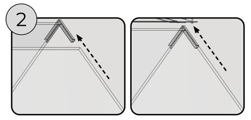
Line up the glass with the glass clip, and carefully push into place. The glass clips can be loosened on both sides to allow easier fitting.
